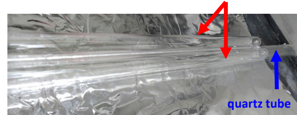
Hg lamp consisting of two connected ampoules
